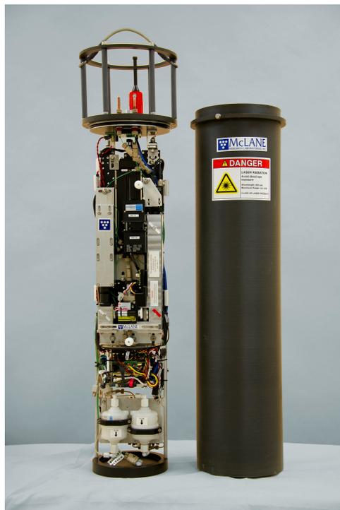
Figure 5: The FlowCytobot system and this external protection tube.
